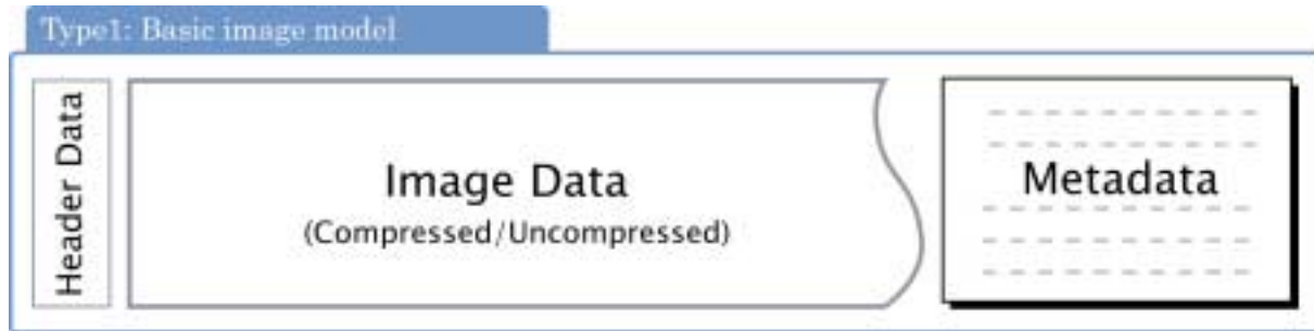
Figure 2-2: Basic conceptual structure of a digital image
