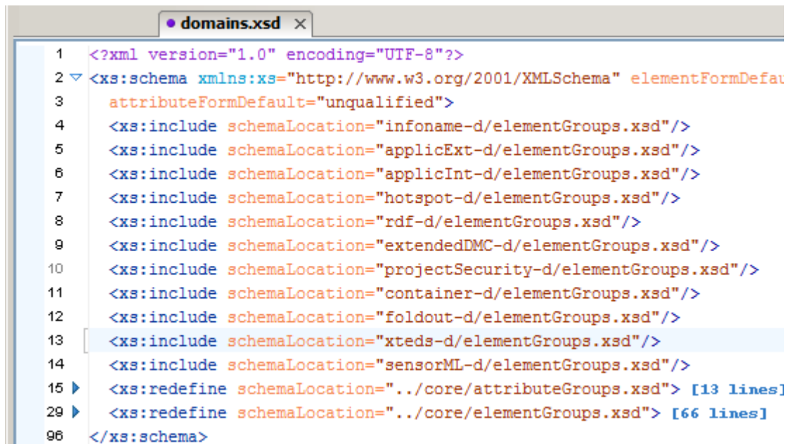
Figure 10: Content of the schema domains.xsd (here including S1000D and non S1000D domains such as xteds and sesorML )
