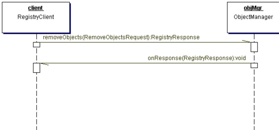
Figure 14: Remove Objects Sequence Diagram
