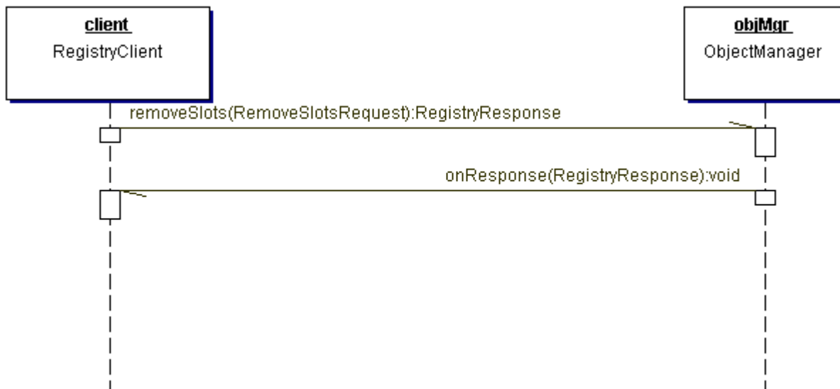
Figure 11: Remove Slots Sequence Diagram
