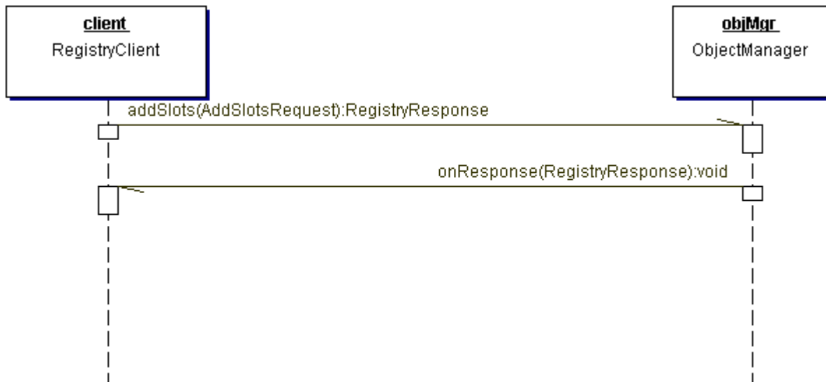
Figure 10: Add Slots Sequence Diagram
