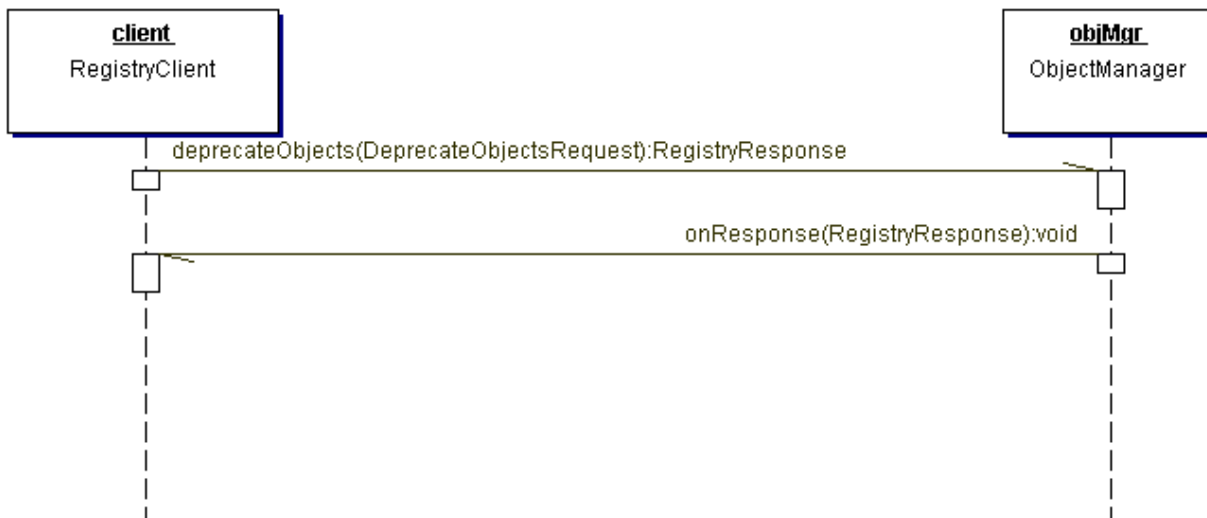
Figure 13: Deprecate Objects Sequence Diagram
