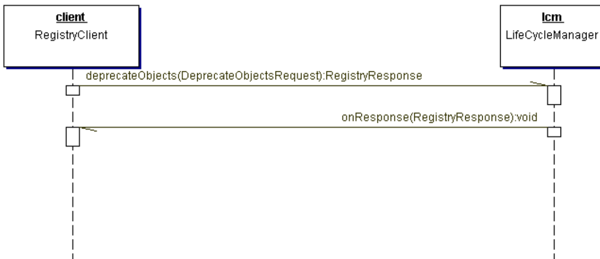
Figure 12: Deprecate Objects Sequence Diagram
