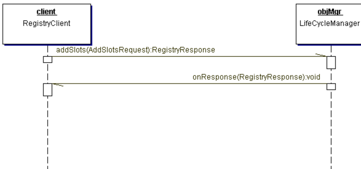
Figure 9: Add Slots Sequence Diagram
