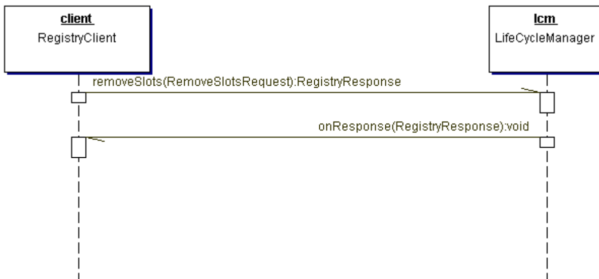
Figure 10: Remove Slots Sequence Diagram
