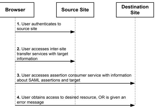
Two HTTP-based techniques are used in the web browser SSO profiles for conveying information from one site to another via a standard commercial browser.
