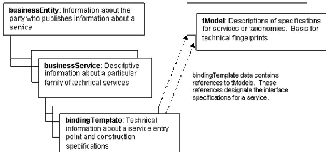
Services are represented in UDDI by the businessService data structure, and the details of how and where the service is accessed are provided by one or more bindingTemplate structures. The businessService might be thought of as a logical container of services. The bindingTemplate structure contains the accessPoint of the service, as well as references to the tModels it is said to implement.
