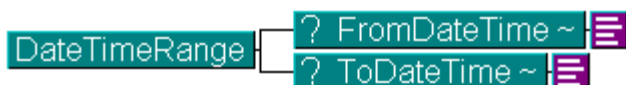
Figure F.k: The DateTimeRange structure provides a date or time range relative to a transaction or structure within a transaction.
