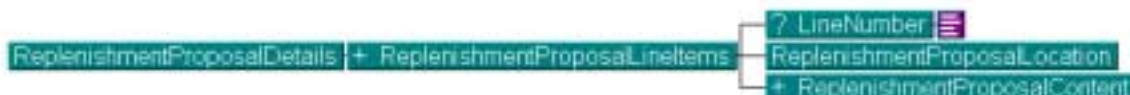
Figure 8.10.2.d: ReplenishmentProposalDetails contains product, quantity, location, and timing details per line item of the replenishment proposal response.
