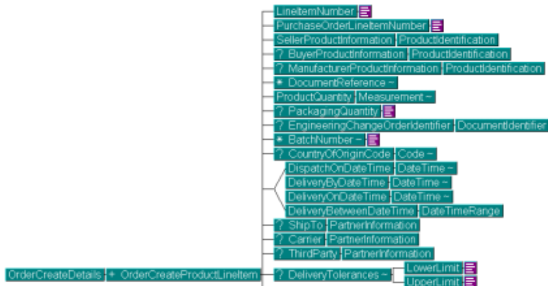
Figure 5.3.2.d: OrderCreateDetails structure (part 1)
