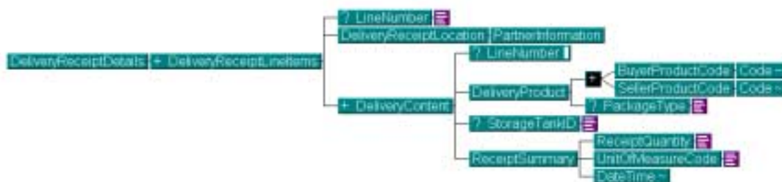
Figure 8.15.2.d: DeliveryReceiptDetails contains product, quantity, location, and timing details per line item of the transaction.
