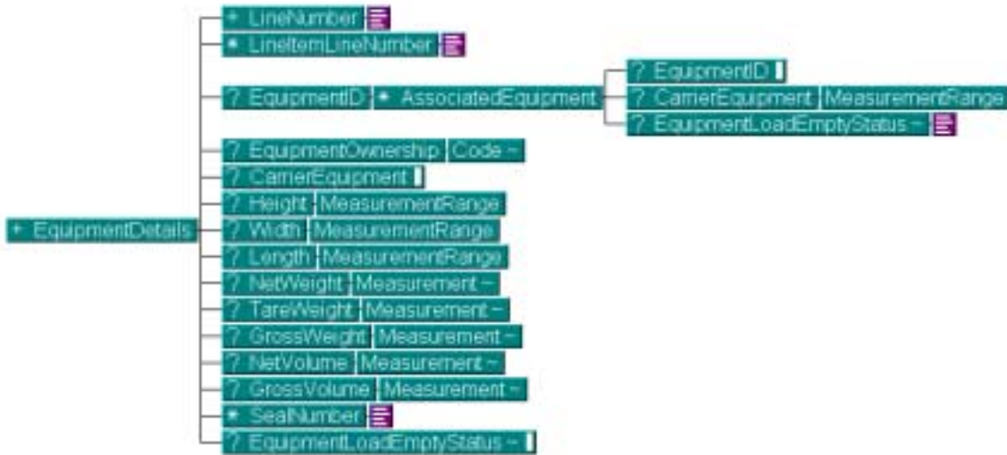
Figure 5: This shows the structure of the Equipment Detail used to specify the equipment requirements.
