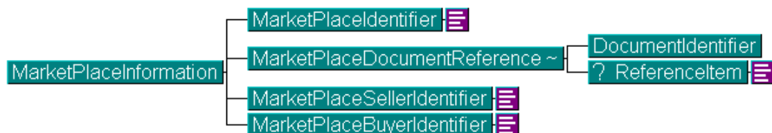
Figure F.u: The MarketPlaceInformation structure identifies a MarketPlace, the buyer and the seller. This structure also includes a MarketPlaceDocumentReference which identifies additional MarketPlace references for a transaction.
