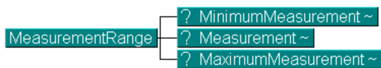
Figure F.w: The MeasurementRange structure identifies a measurement range within a transaction. This structure allows for a minimum and/or maximum measurement as well as an average measurement.
