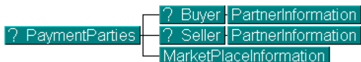
Figure 7.4.2.c: The PaymentPartners are the Buyer, Seller, and Marketplace address and contact information for the parties to the transaction.
