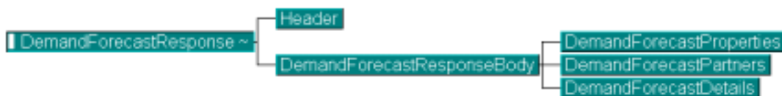
Figure 8.4.2.a: DemandForecastResponse structure to be used for receipt confirmation of demand forecasting transactions
