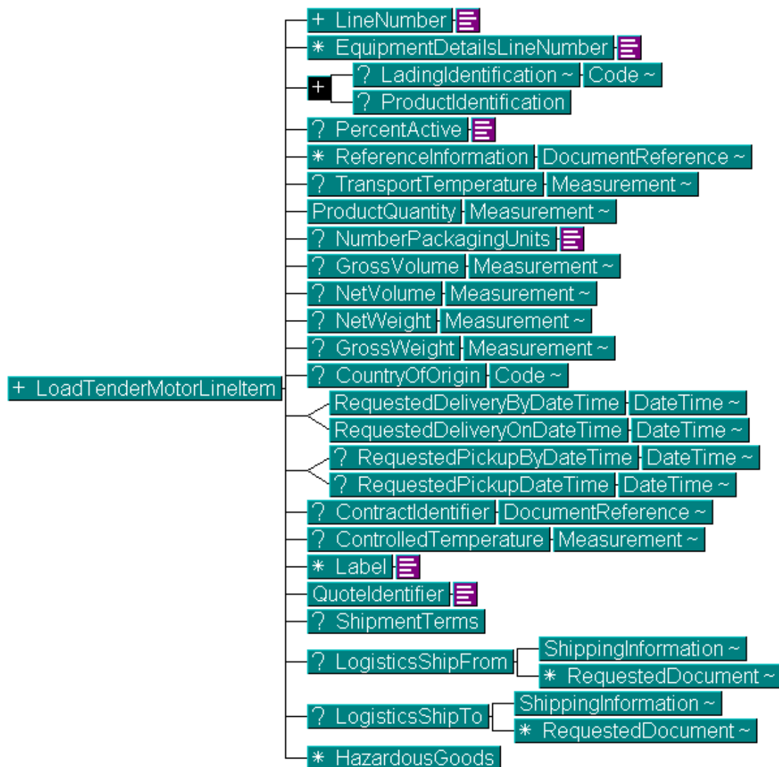
Figure 6: Load Tender MotorLineItem information is used to communicate the details of shipment.
