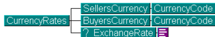
Figure F.h: The CurrencyRates structure.
