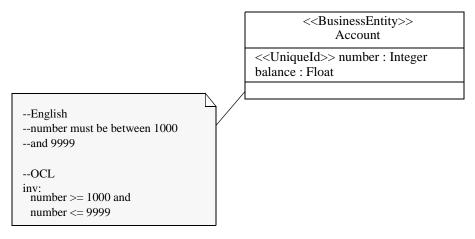
Figure 7 Platform-Independent Model, Enhanced with Stereotypes
