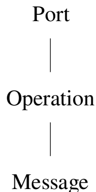
Figure 1 - WSDL 1.1 hierarchical data model
