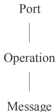
Figure 1 - WSDL 1.1 hierarchical data model
